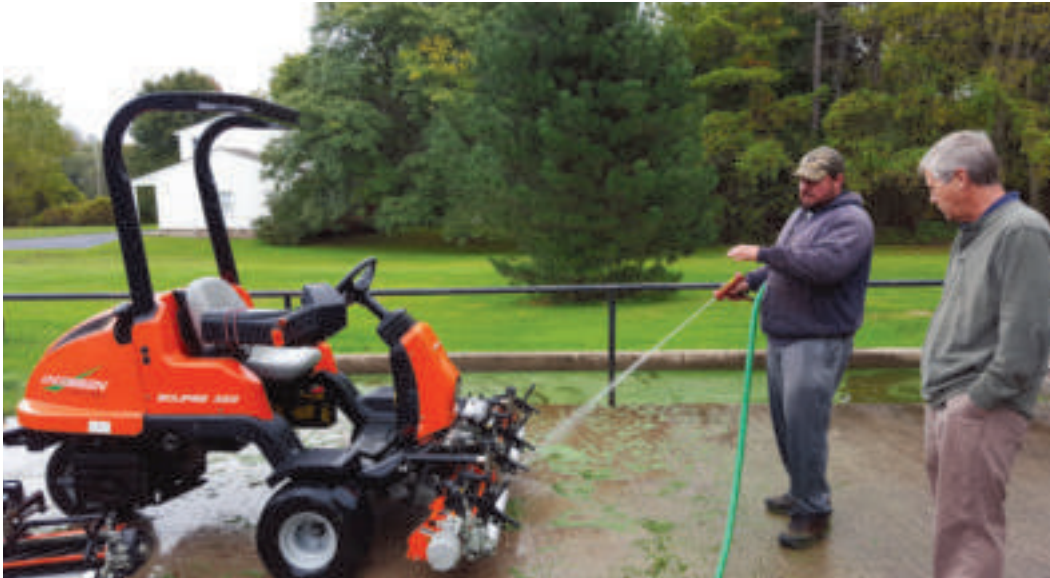
Locust Hill: Rick Slattery, right, Locust Hill golf course superintendent, and Casey Grann, senior assistant, worked with P2I to find a way to recycle wastewater when washing mowers. Right: P2I engineers identified flow restrictors and nozzles that reduced water flow without affecting quality.
