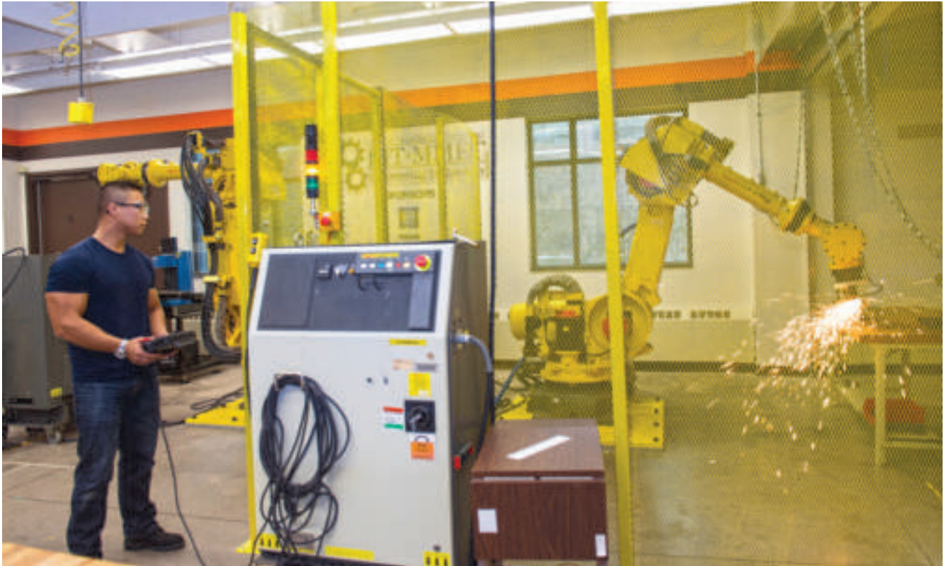
Manufacturing Process: SunWoo Ji uses the Fanuc R-2000iA/210F robots as part of a welding process where the robots interface with programmable logic controllers and vision systems to enable a fully automated welding operation.
