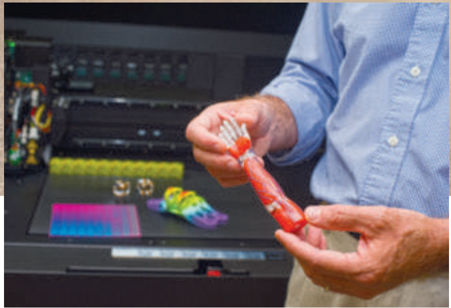
Making Models: Denis Cormier, director of the center, holds a 3D-printed model of an arm that could be used as a guide to assist orthopedic surgeons during reconstruction surgeries.
