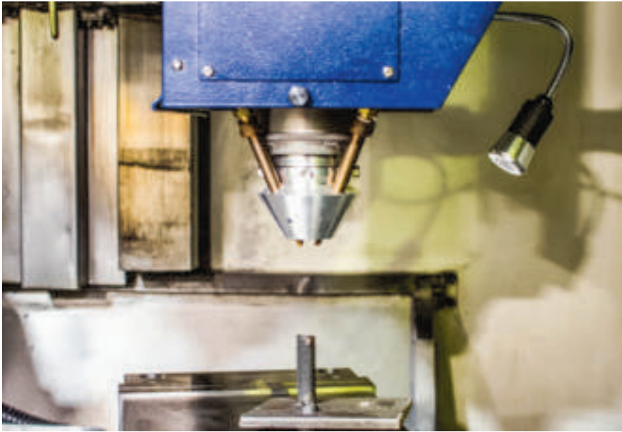
Remanufacturing: The additive manufacturing cell in GIS remanufactures components and prototype designs for future products. GIS uses this equipment when working with military and industrial partners.
